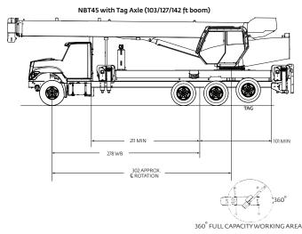
Configuration 4: Extended T-box 31,39 m (103 ft), 38,71 m (127 ft) or 43,29 m (142 ft) Boom with Tag Axle
