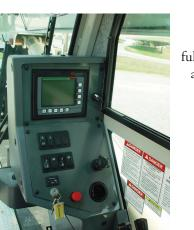
(LMI) is standard on all NBT45 machines. The LCD display is visible in full or low light and displays all crane load lifting values simultaneously. Includes Work Area Definition System (WADS).
