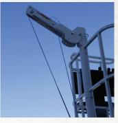
Narrow Outrigger Spread An 8 foot spread provides full 360 degree operation, allowing setup in areas as tight as a single parking stall
