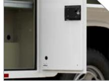
**H** Features double-shell, 20-gauge, two-sided A-40 galvaneal steel compartment doors
