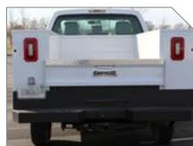
**M** Includes slam-lock tailgate with one-hand center release
