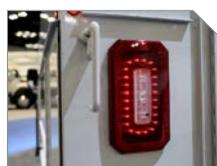
**N** Upgraded surface mount lighting system features LED S/T/T and B/U, LED strobe option\* with (8) selectable patterns, and built-in reflectivity for additional safety\*\*
