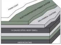
**A** Features 14-gauge, two-sided A-40 galvaneal steel shell
