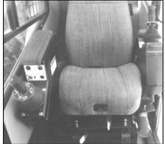
*National gives you a choice of two standard in-the-cab controls for the Series 1500 telescoping crane. Unless you specify otherwise, the crane will be equipped with the single axis, dual lever control shown above left. You may, at no extra charge, specify the dual axis, single lever joystick (“wobble stick” style), shown above right.*
