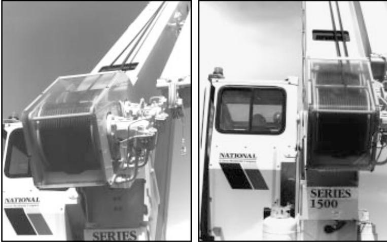
All winch pulls and speeds are shown on the fifth layer. Winch line pulls would increase on the first, second, third and fourth layers. Winch line speeds would decrease on the first, second, third and fourth layers. Winch line pulls may be limited by winch capacity or the cable safety factor shown below.
