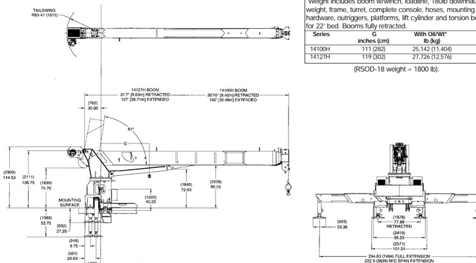
\*Weight includes boom w/winch, loadline, 180lb downhaul weight, frame, turret, complete console, hoses, mounting hardware, outriggers, platforms, lift cylinder and torsion box for 22' bed. Booms fully retracted.
