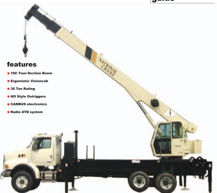
The mounting configuration shown is based on an 85% stability factor. The complete unit must be installed on the truck in accordance with factory requirements, and a test performed to determine actual stability and counterweight requirements, since individual truck chassis vary. If bare truck weights are not met, counterweight will be required. A summary of mounting and truck requirements are:
