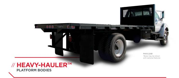
The Heavy-Hauler<sup>™</sup> (PHH) is Knapheide's most rugged platform, designed to handle the most severe of hauling applications. It has been engineered to work in both hoist and non-hoist applications.
